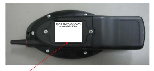
Label with **FCC ID:2AAEP-MSENSOR01** and **IC:11128A-MSENSOR01** will be located at the rear side panel. The statement according to FCC part 15 §15.19(a)(3) is placed in User Manual, page 53 (Application exhibit User\_manual\_24194).
