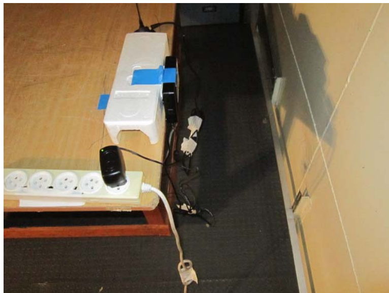
Photograph 8.1.2 Setup for conducted emissions measurements
