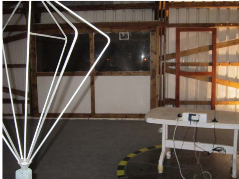
Photograph 8.2.5 Setup for final radiated emission measurements, EUT cabling
