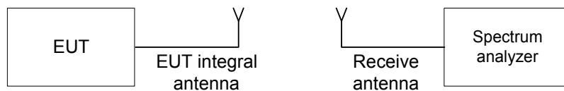
Figure 7.1.1 Setup for transmitter shut down test
