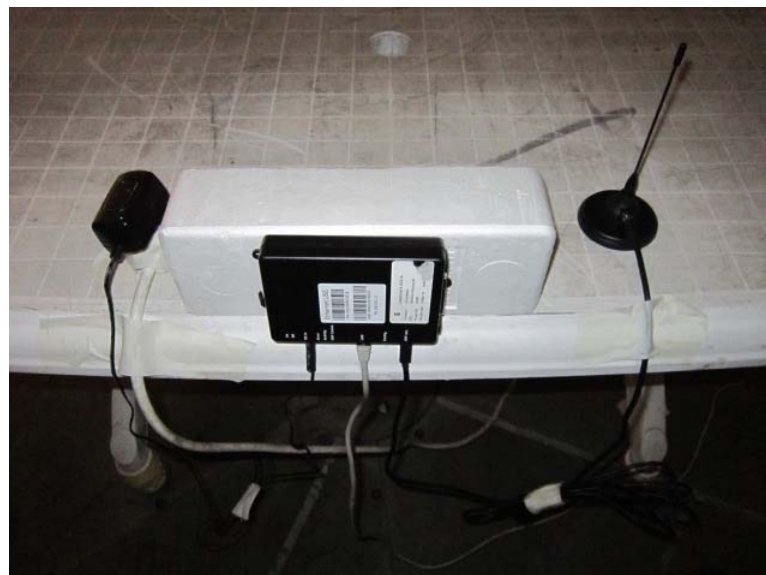
Photograph 8.2.5 Setup for final radiated emission measurements, EUT cabling
