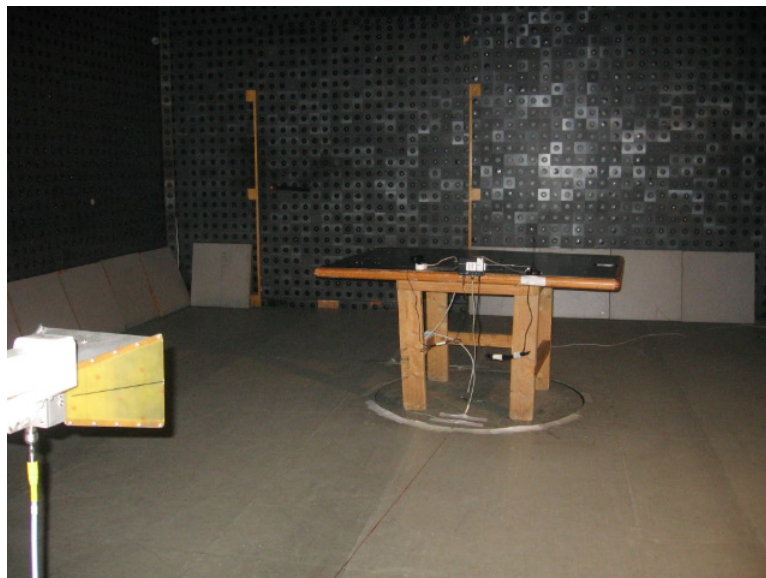
Photograph 8.2.2 Setup for radiated emission measurements
