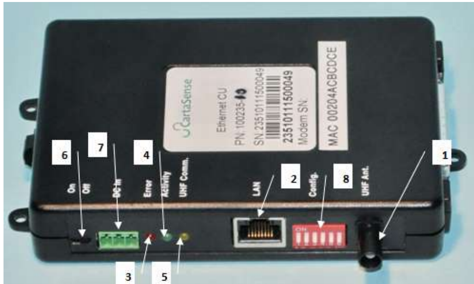
Figure 8: Ethernet U-Sensor Gateway
