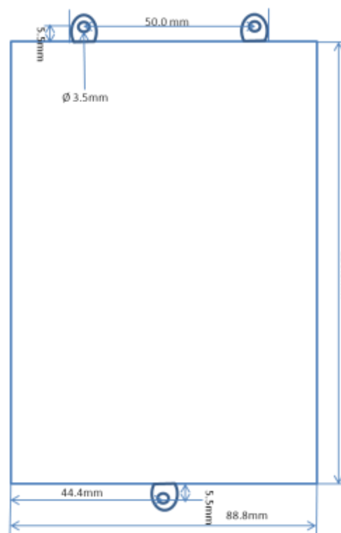
Figure 11: USG mount drill scheme
