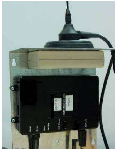
Figure 15: RS with USG and UHF Antenna using single mounting
