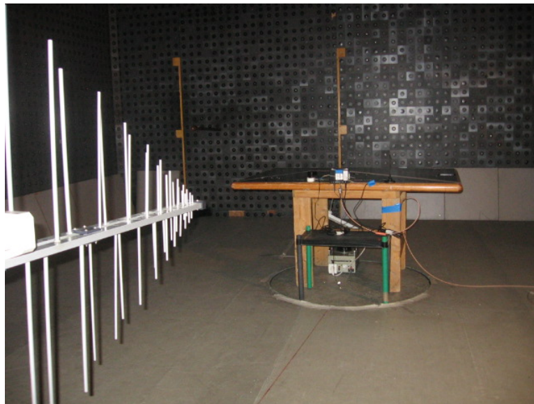
Photograph 8.2.1 Setup for radiated emission measurements
