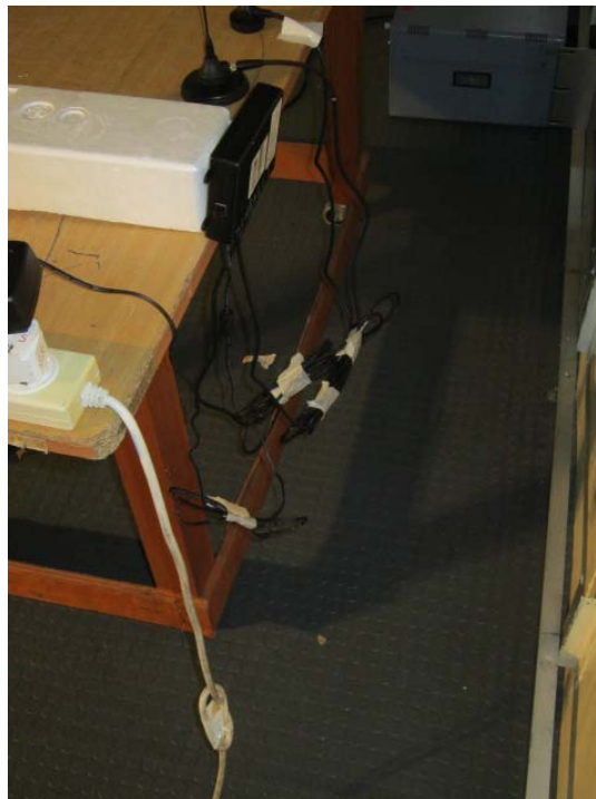
Photograph 8.1.2 Setup for conducted emissions measurements
