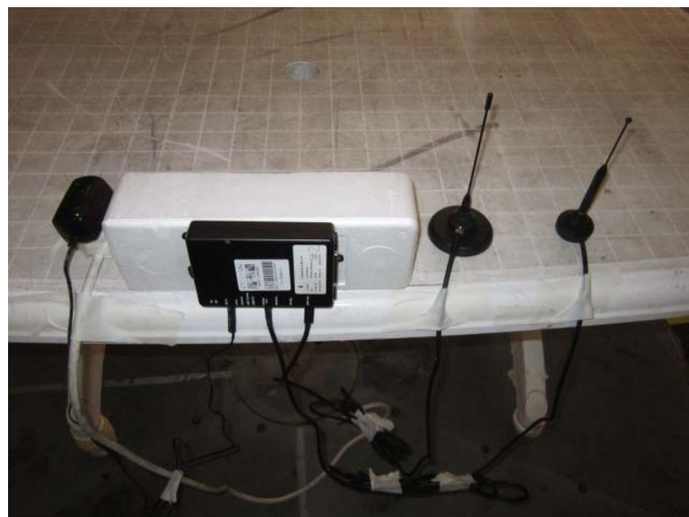
Photograph 8.2.4 Setup for radiated emission measurements, EUT cabling
