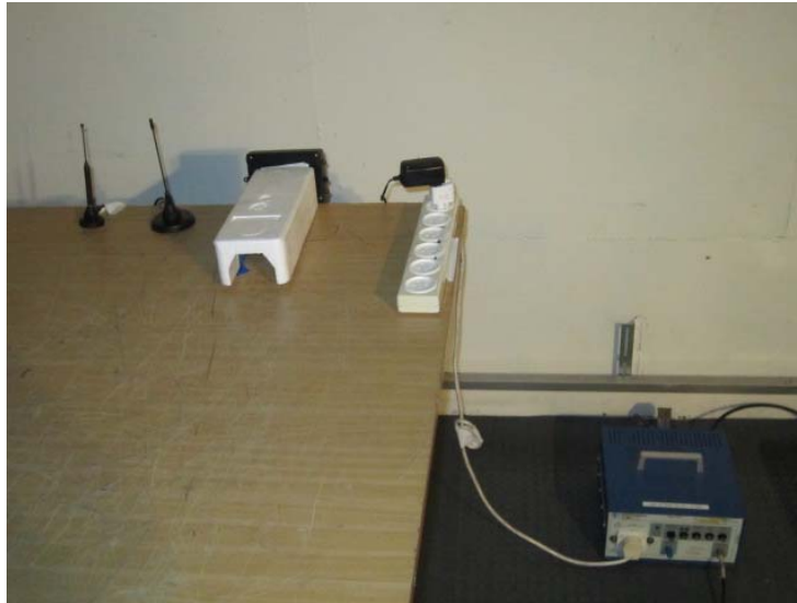
Photograph 8.1.2 Setup for conducted emissions measurements
