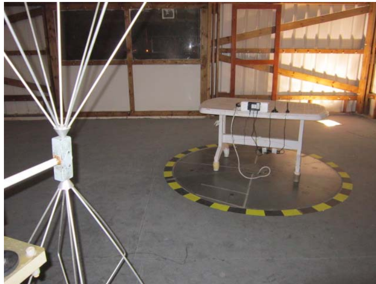
Photograph 8.2.3 Setup for radiated emission measurements, general view
