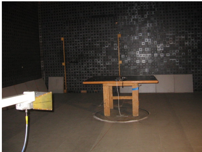
Photograph 8.2.1 Setup for radiated emission measurements
