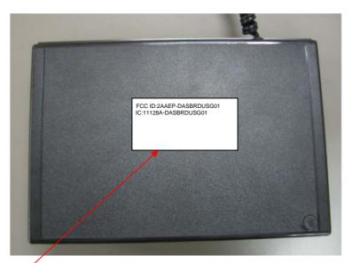
Label with FCC ID:2AAEP-DASBRDUSG01 and IC:11128A-DASBRDUSG01 will be located at the rear side panel. The statement according to FCC part 15 §15.19(a)(3) is placed in User Manual, page 53 (Application exhibit User\_manual\_24191).
