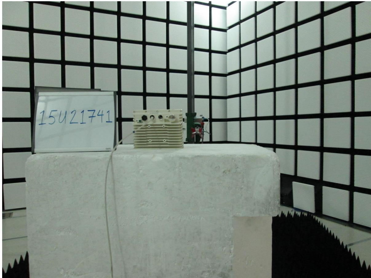
RADIATED RF - BACK PHOTO (ABOVE 1GHz)
