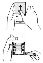
2. Install or replace the 4 AA batteries, Make the battery positive (+) and negative (-) extremely consistent with the marks in the battery box, and then close the battery cover.
