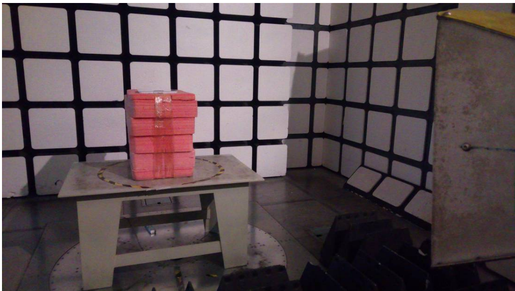
Radiated Emissions View (Above 1 GHz)
