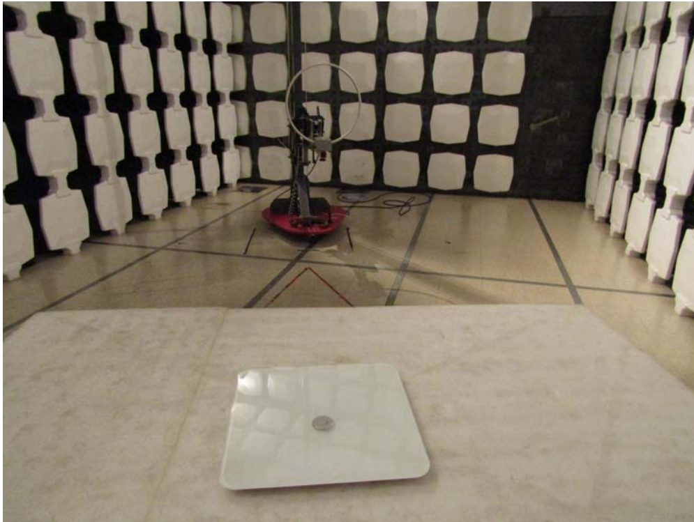
Measurement of Radiated Emission Test Set Up
