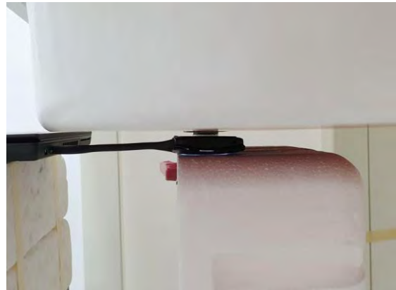
Fig.4 EUT Back side to flat phantom
