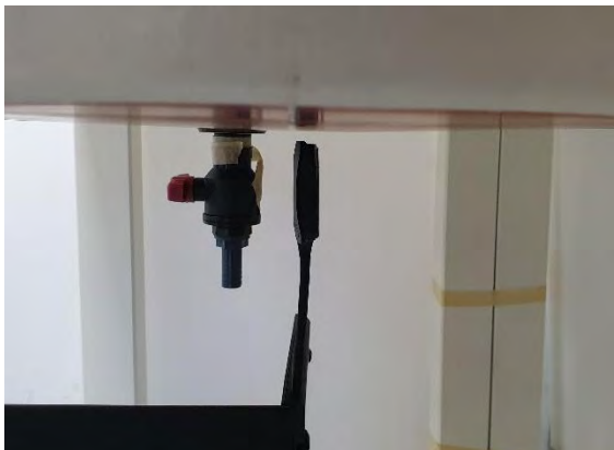
Fig.5 EUT Top side to flat phantom
