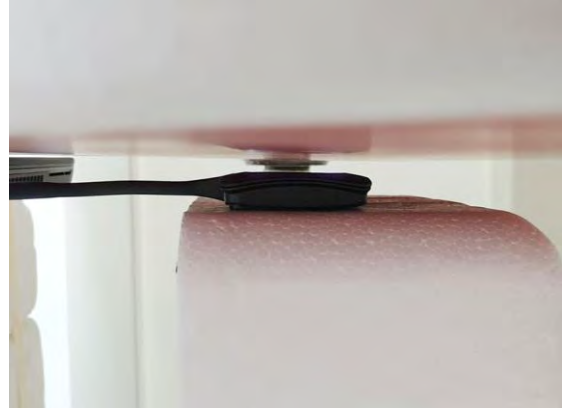
Fig.3 EUT Front side to flat phantom
