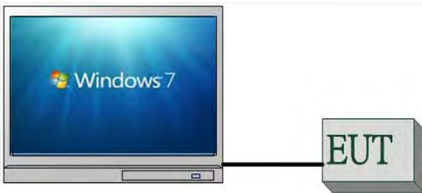
Fig. 2-1 Conducted & Radiated Emission Configuration
