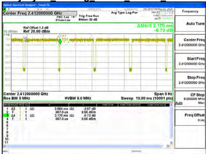
Duty Cycle 802.11g 20MHz Chain1 2412MHz
