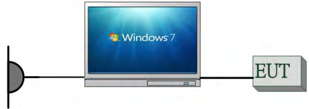
Fig. 2-2 Conducted Emission (AC Power Line) Configuration
