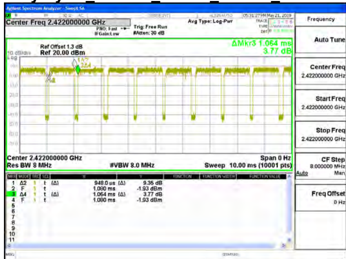
Duty Cycle 802.11n 40MHz Chain1 2422MHz
