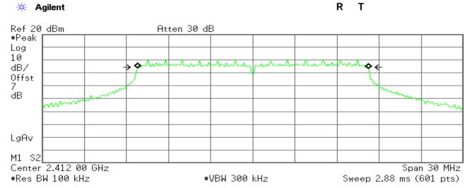
Occupied Bandwidth 16.4585 MHz Occ BW % Pwr 99.00 % x dB -6.00 dB
