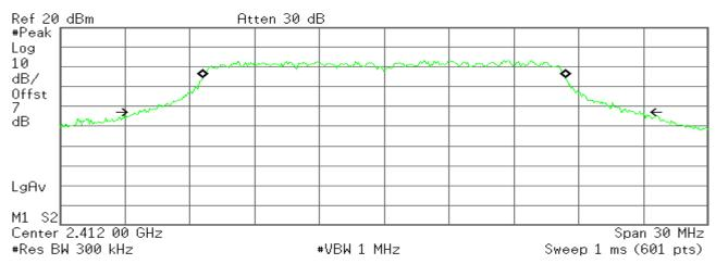
Occupied Bandwidth 16.7670 MHz Occ BW % Pwr 99.00 % x dB -26.00 dB
