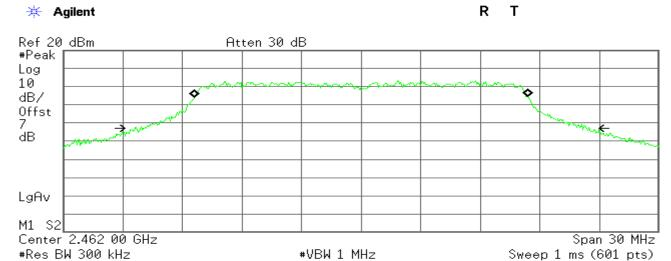
Occupied Bandwidth 16.7751 MHz Occ BW % Pwr 99.00 % x dB -26.00 dB
