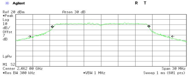
Occupied Bandwidth 16.8993 MHz Occ BW % Pwr 99.00 % x dB -26.00 dB
