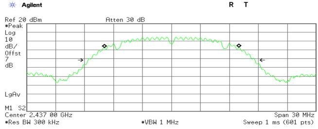
Occupied Bandwidth 13.9538 MHz Occ BW % Pwr 99.00 % **x dB** -26.00 dB
