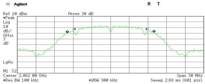
Occupied Bandwidth 13.9435 MHz Occ BW % Pwr 99.00 % x dB -6.00 dB
