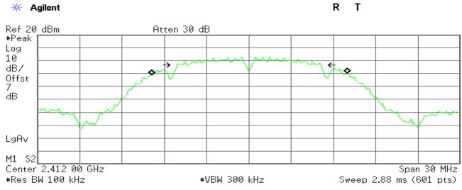
Occupied Bandwidth 13.9102 MHz Occ BW % Pwr 99.00 % x dB -6.00 dB
