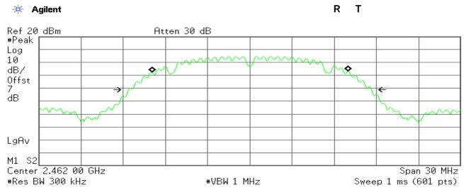
Occupied Bandwidth 13.9437 MHz Occ BW % Pwr 99.00 % x dB -26.00 dB
