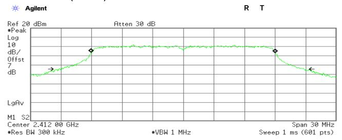
Occupied Bandwidth 17.9812 MHz Occ BW % Pwr 99.00 % **x dB** -26.00 dB
