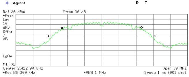
Occupied Bandwidth 13.9562 MHz Occ BW % Pwr 99.00 % x dB -26.00 dB
