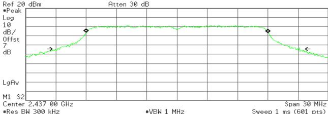
Occupied Bandwidth 18.0017 MHz Occ BW % Pwr 99.00 % x dB -26.00 dB
