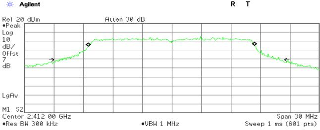
Occupied Bandwidth 16.9008 MHz Occ BW % Pwr 99.00 % x dB -26.00 dB
