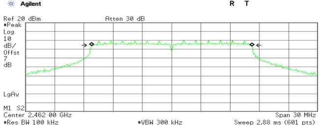
Occupied Bandwidth 16.4480 MHz Occ BW % Pwr 99.00 % x dB -6.00 dB
