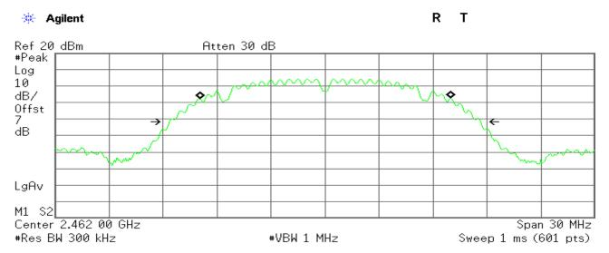
Occupied Bandwidth 13.9468 MHz Occ BW % Рыг 99.00 % х dB -26.00 dB
