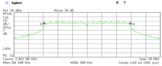
Occupied Bandwidth 17.6383 MHz 0cc BW % Pwr 99.00 % x dB -6.00 dB
