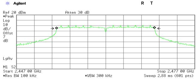
Occupied Bandwidth 16.4486 MHz 0cc BW % Pwr 99.00 % x dB -6.00 dB
