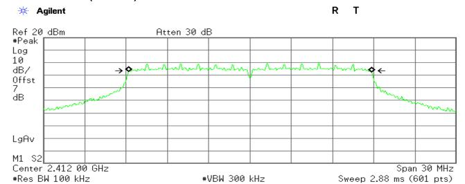
Occupied Bandwidth 17.6426 MHz Occ BW % Pwr 99.00 % × dB -6.00 dB
