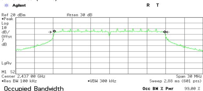
Transmit Freq Error 16.274 kHz x dB Bandwidth 17.360 MHz
