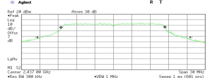
Occupied Bandwidth 16.9563 MHz Occ BW % Pwr 99.00 % x dB -26.00 dB
