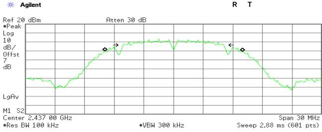
Occupied Bandwidth 13.9444 MHz Occ BW % Pwr 99.00 % x dB -6.00 dB
