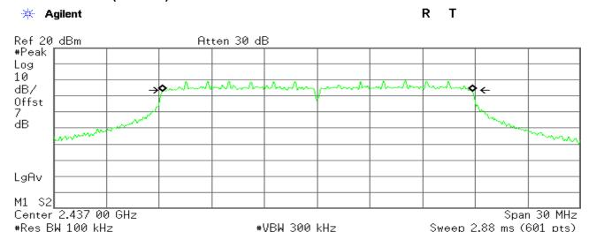
Occupied Bandwidth 17.6532 MHz Occ BW % Pwr 99.00 % -6.00 dB x dB
