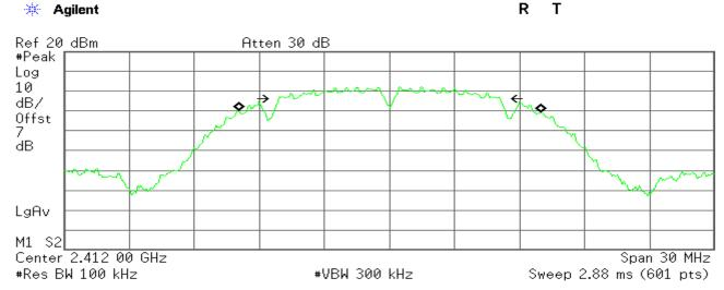
Occupied Bandwidth 13.9618 MHz Occ BW % Pwr 99.00 % -6.00 dB x dB
