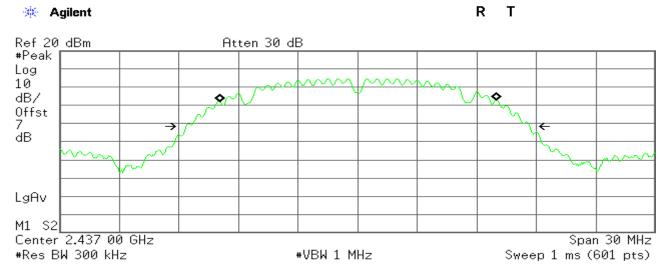
Occupied Bandwidth 13.9563 MHz Occ BW % Pwr 99.00 % x dB -26.00 dB
