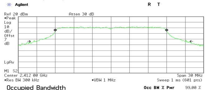
Transmit Freq Error 1.838 kHz x dB Bandwidth 24.733 MHz
