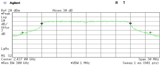
Occupied Bandwidth 17.9696 MHz Occ BW % Pwr 99.00 % x dB -26.00 dB
