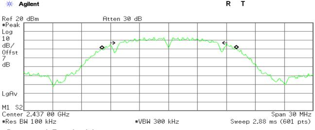
Occupied Bandwidth 13.9395 MHz Occ BW % Pwr 99.00 % x dB -6.00 dB
