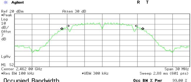
Occupied Bandwidth 13.8752 MHz Occ BW % Pwr 99.00 % x dB -6.00 dB
