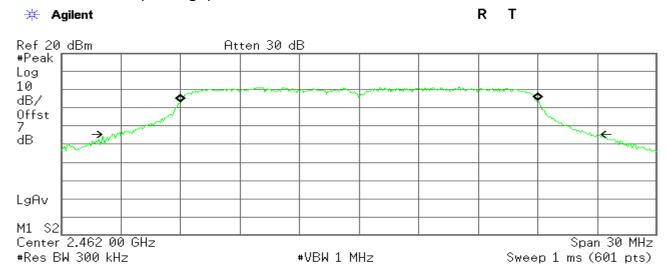
Occupied Bandwidth 17.9679 MHz Occ BW % Pwr 99.00 % x dB -26.00 dB
