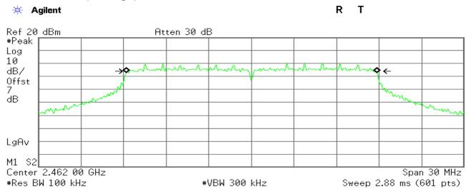
Occupied Bandwidth 17.6554 MHz Occ BW % Pwr 99.00 % x dB -6.00 dB
