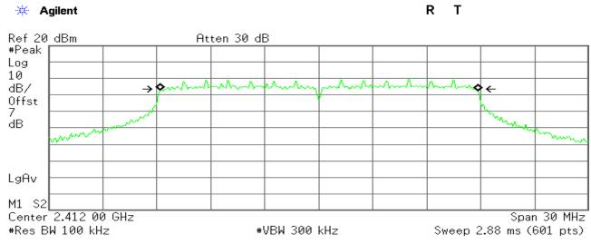
Occupied Bandwidth 17.6474 MHz Occ BW % Pwr 99.00 % x dB -6.00 dB
