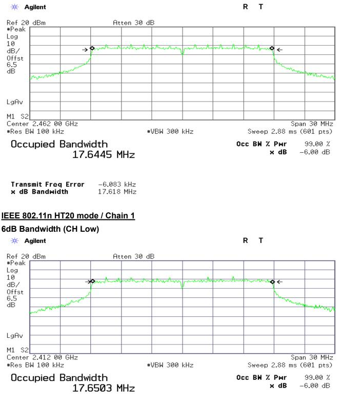
Transmit Freq Error 15.412 kHz x dB Bandwidth 17.317 MHz
