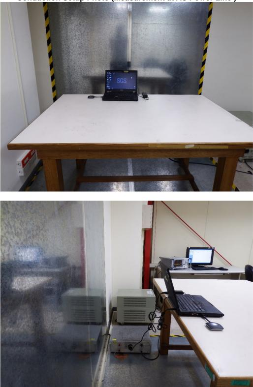
Conduction Setup Photo (Measurement at AC Power Line )
