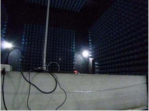
Radiated Emission Set up Photos (Below 1GHz)
