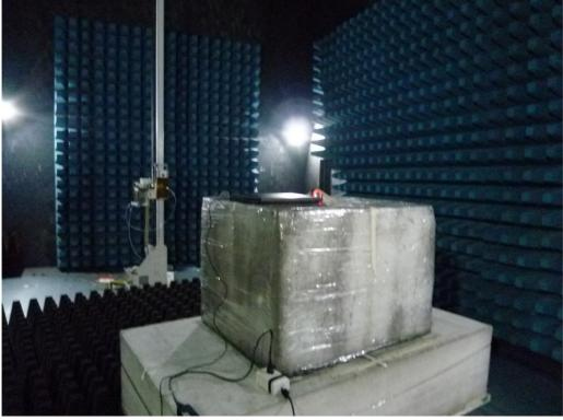
**Radiated Emission Set up Photos (Front View)**
