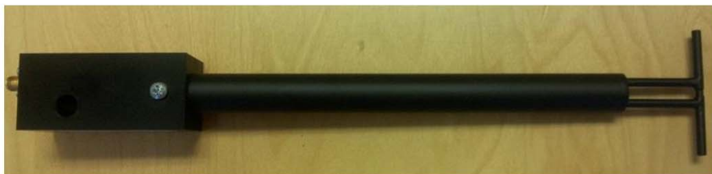
Figure 1 – MVG COMOSAR Validation Dipole
