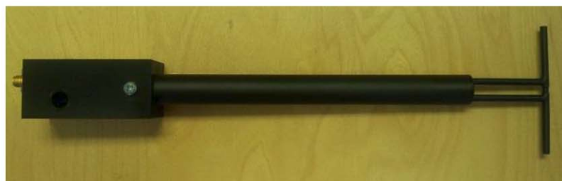
Figure 1 – MVG COMOSAR Validation Dipole
