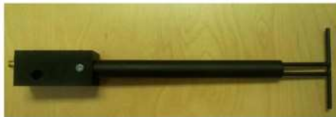
Figure 1 – MVG COMOSAR Validation Dipole
