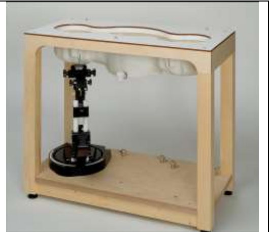
Fig. 8.7 Photo of SAM Twin Phantom
