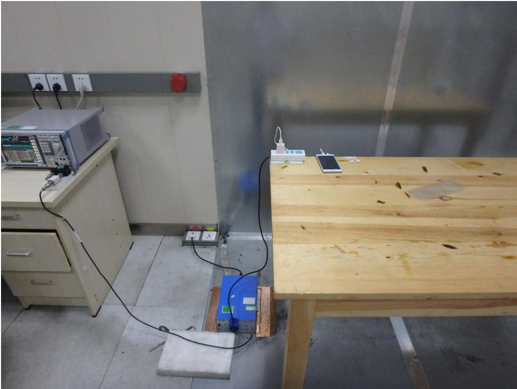
FCC RADIATED EMISSION TEST SETUP
