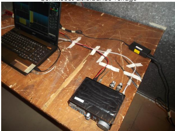
Continuous disturbance voltage
