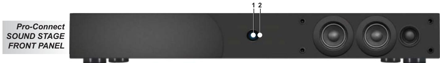
**1. STATUS LED** - (Behind front panel lens.) One multi-color LED. This LED will illuminate red/blue and flash in different modes to indicate changes in the SOUND STAGE operational status. SOLID RED - OFF (Standby). Power cord is connected and AC switch is turned ON, but the SOUND STAGE is OFF.
