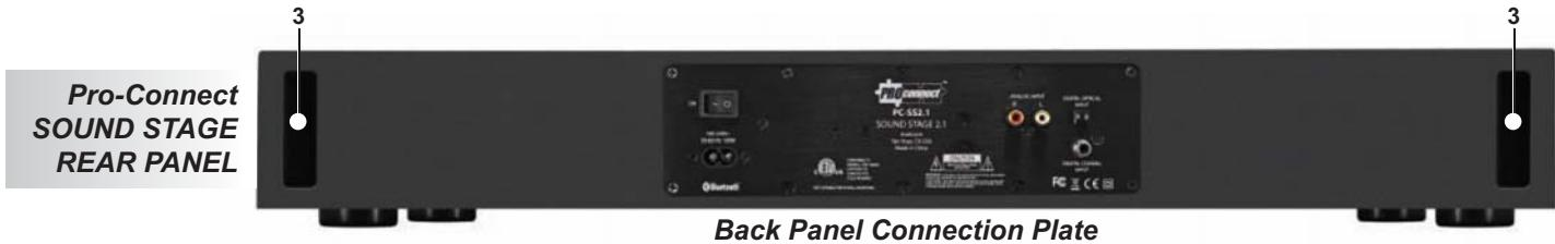
**3. FRONT AND REAR PANEL BASS PORTS** - Two pairs of tuned openings in the SOUND STAGE cabinet allow air to 'release' from the cabinet and enhance low frequency audio. Allow at least 3 inches of clearance to a back wall to allow air to move freely from the ports for full bass extension.
