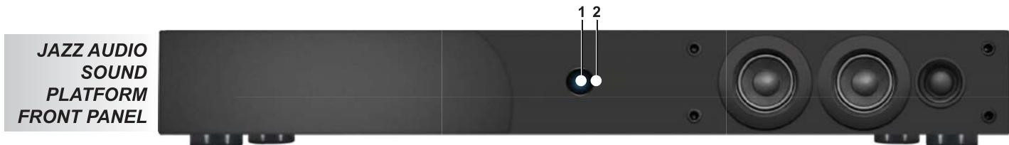
**1. STATUS LED** - (Behind front panel lens.) One multi-color LED. This LED will illuminate red/blue and flash in different modes to indicate changes in the SOUND PLATFORM operational status. SOLID RED - OFF (Standby). Power cord is connected and AC switch is turned ON, but the SOUND PLATFORM is OFF.
