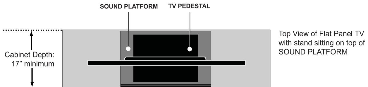
The cabinet top should be at least seventeen inches deep to properly support the SOUND PLATFORM. The SOUND PLATFORM is sixteen and a half inches deep (with grille attached) and extra space will be required between the SOUND PLATFORM and a wall behind the cabinet for cables connecting the SOUND PLATFORM to the TV or other A/V sources (3 inches minimum).
