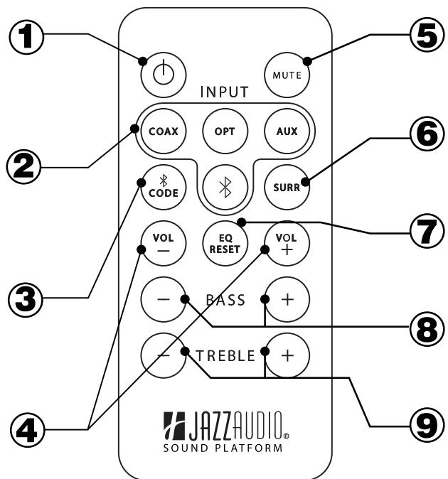
**1. POWER** - Press this button to turn the SOUND PLATFORM ON/OFF.
