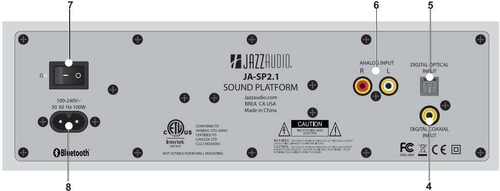
**5. DIGITAL OPTICAL INPUT** - One TOSLINK® connector. Connect to the Digital Optical OUT on a TV or other source. This input is selected by pressing the OPT button on the SOUND PLATFORM IR Remote.
