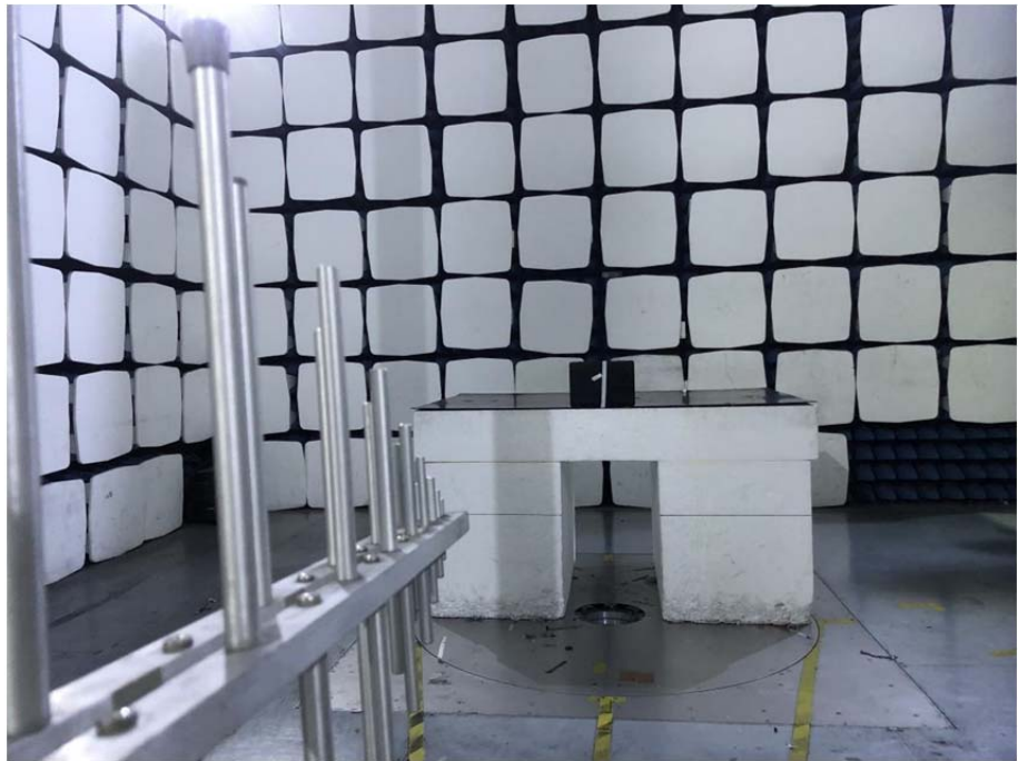
Radiation Emission Test Setup (30MHz to 1GHz)
