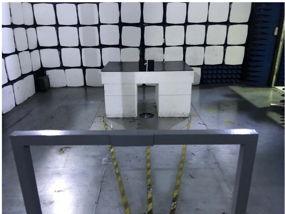
Radiation Emission Test Setup (Below 30MHz)
