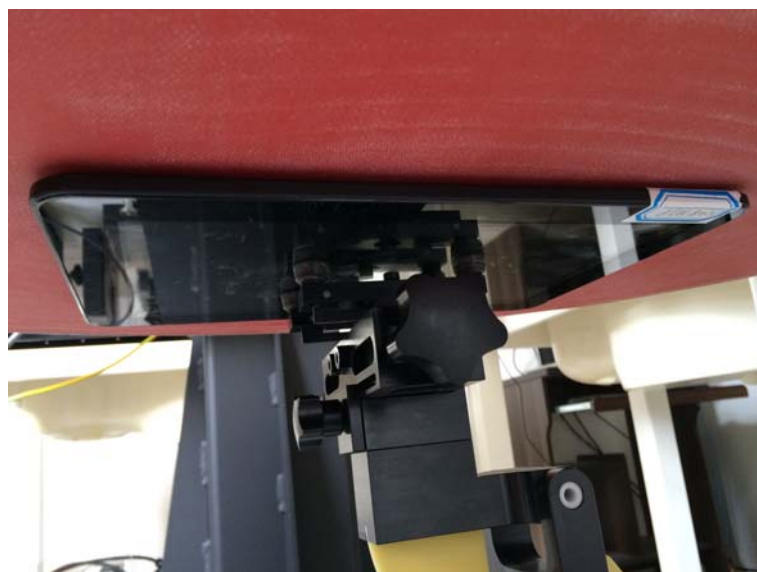
0cm Body-worn Rear Side Setup Photo
