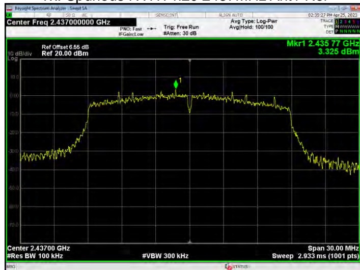
Tx. Spurious NVHT n20 2437MHz Ant1 Emission
