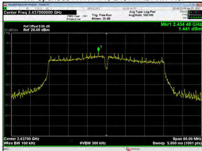
Tx. Spurious NVHT n40 2437MHz Ant1 Emission
