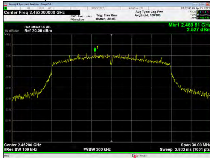
Tx. Spurious NVHT n20 2462MHz Ant1 Emission
