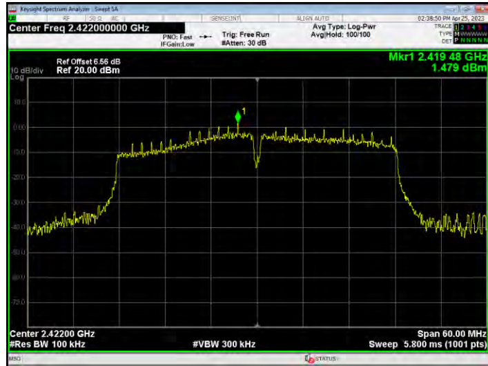
Tx. Spurious NVHT n40 2422MHz Ant1 Emission
