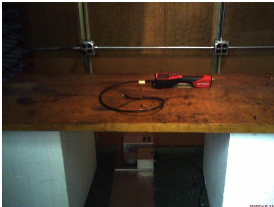
Figure 6: Conducted Emissions Test Setup Photograph(s).
