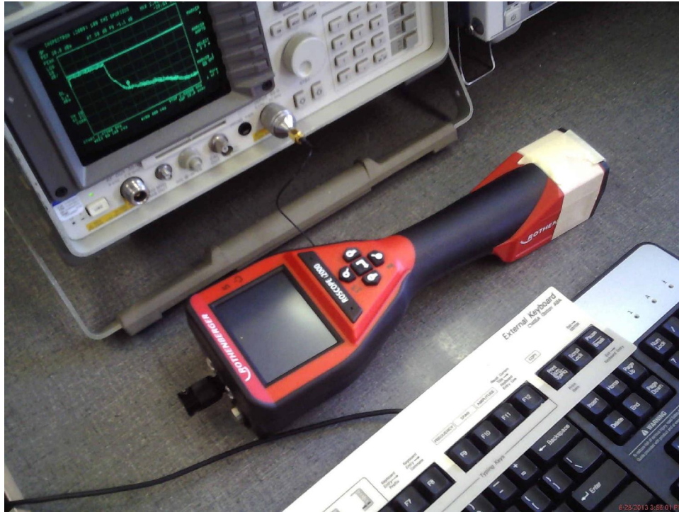
Figure 5: Conducted RF Test Setup Photograph(s).
