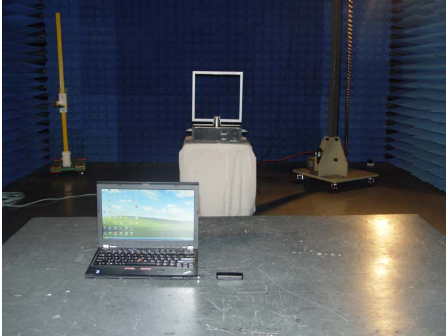
Radiated emissions test 30MHz - 1GHz
