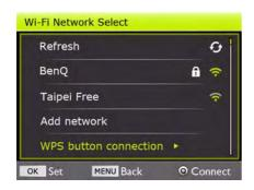
A list of SSIDs will be listed in Wi-Fi Network Select if available. Use 4-way control and press & key to scroll and select Refresh for more SSIDs, your desired SSID, Add network, or WPS button connection.
