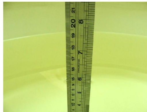
Fig 7.2 Photo of Liquid Height for Body SAR
