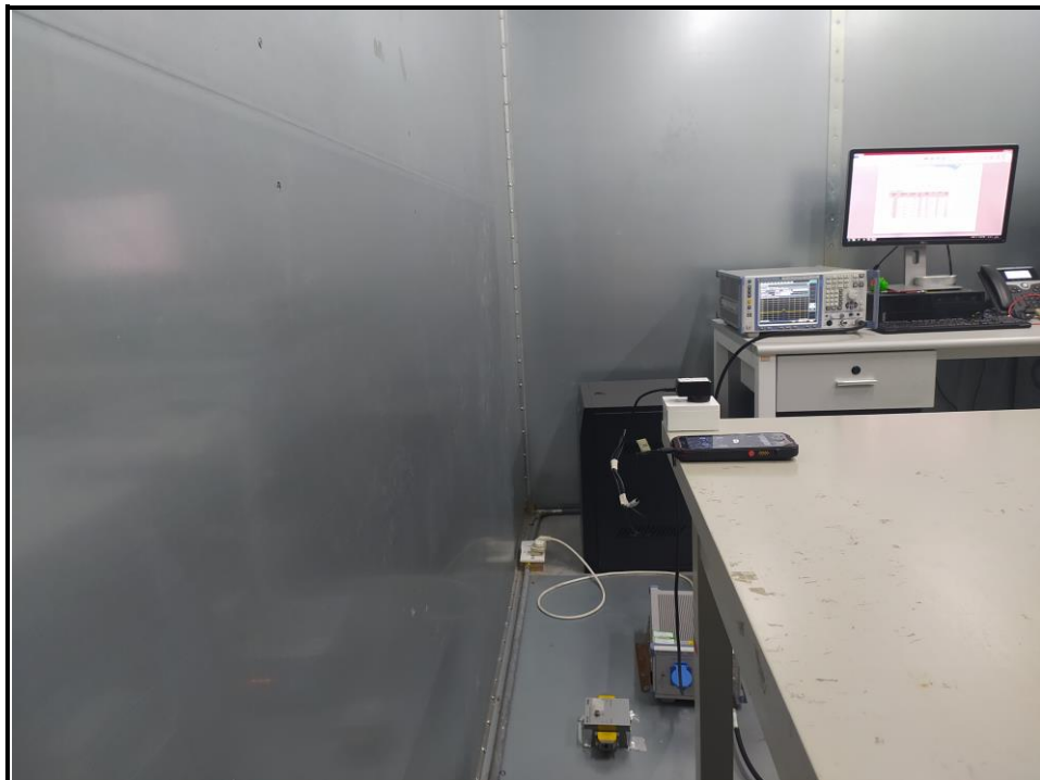
Fig. 4 Power line conducted emission setup photo
