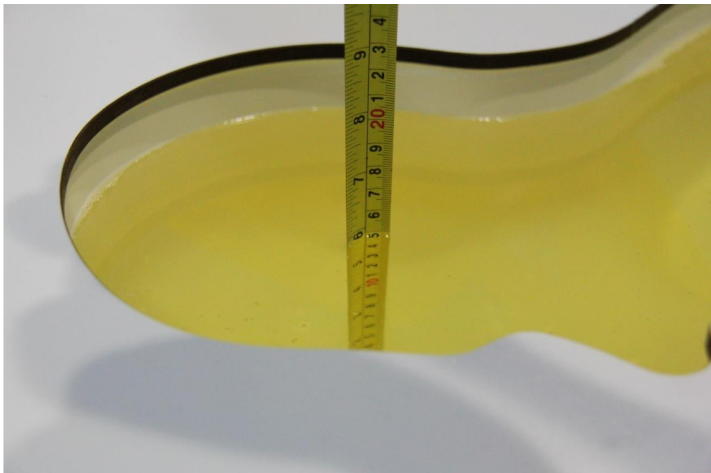
Picture 7-6: Liquid depth in the Head Phantom(2450MHz)
