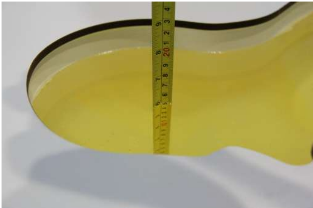
Picture 7-6: Liquid depth in the Head Phantom(2450MHz)
