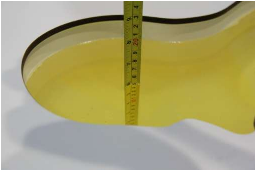
Picture 7-5: Liquid depth in the Head Phantom (2300MHz)
