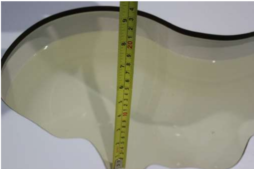
Picture 7-8: Liquid depth in the Head Phantom(5GHz)
