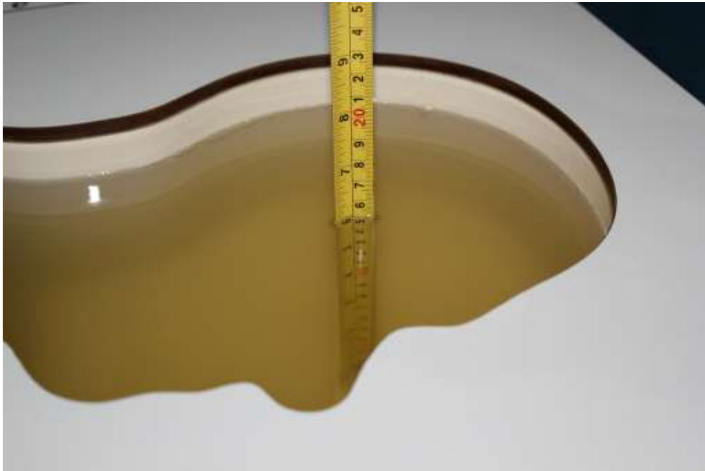
Picture 7-7: Liquid depth in the Head Phantom(2550MHz)
