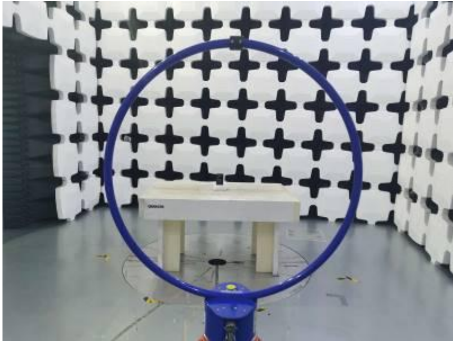
13. Radiated Emissions (Part 15C&E 9kHz-30MHz)
