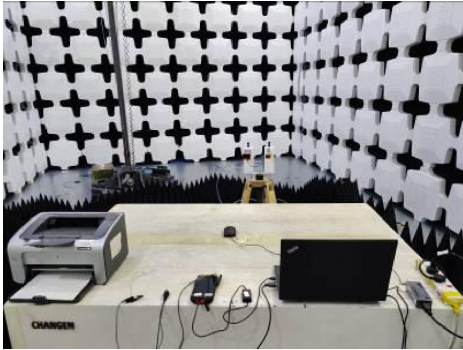
3. Radiated Emissions (Part 15B Data Transfer Mode)(18G-26.5GHz)
