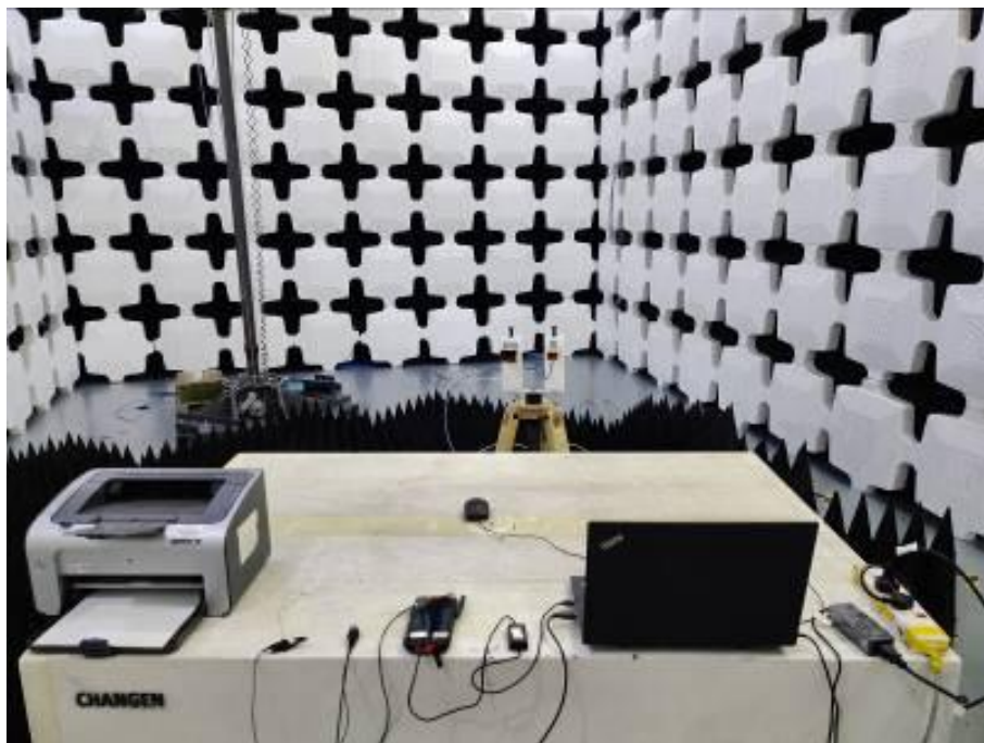
4. Radiated Emissions (Part 15B Data Transfer Mode)(26.5G-30GHz)
