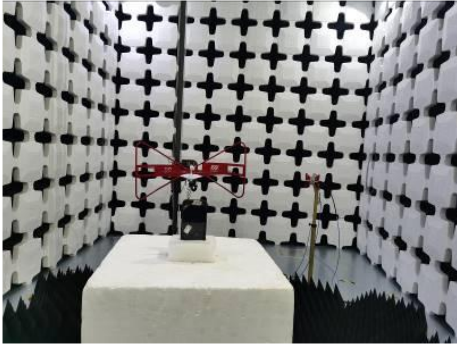
15. Radiated Emissions (Part 15C&E 1G-18GHz)
