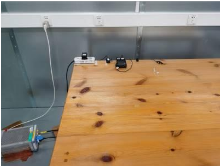
20. Conducted Emission (Part 15B/E Charging mode Type C Wire + Headset)
