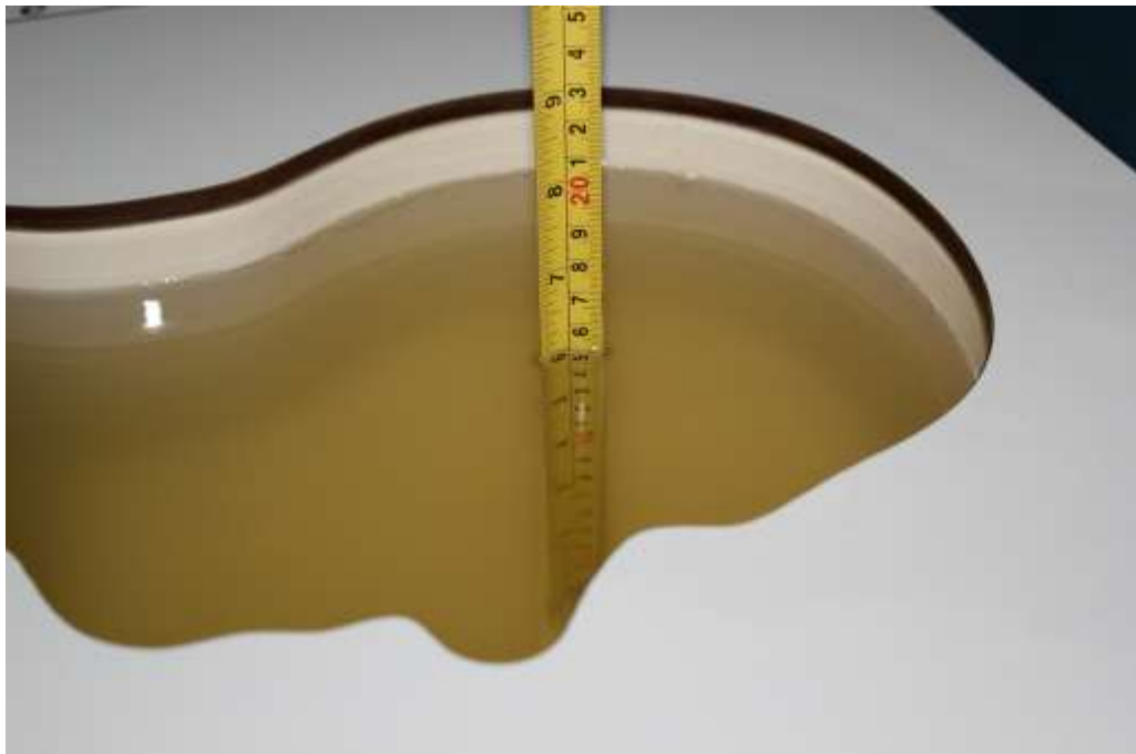
Picture 7-6: Liquid depth in the Head Phantom(2550MHz)
