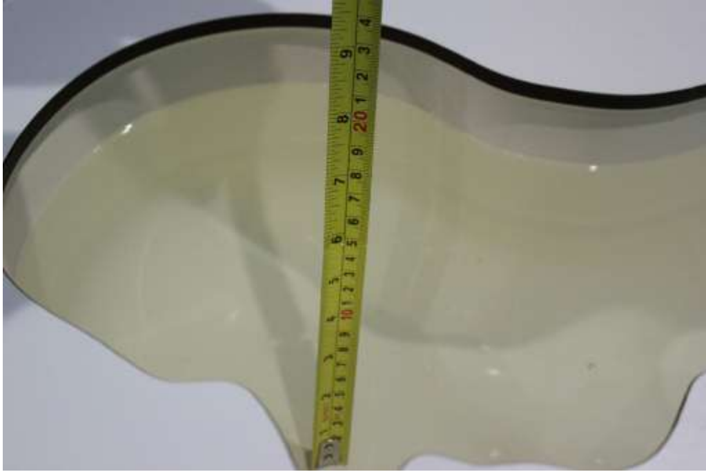
Picture 7-7: Liquid depth in the Head Phantom(5GHz)
