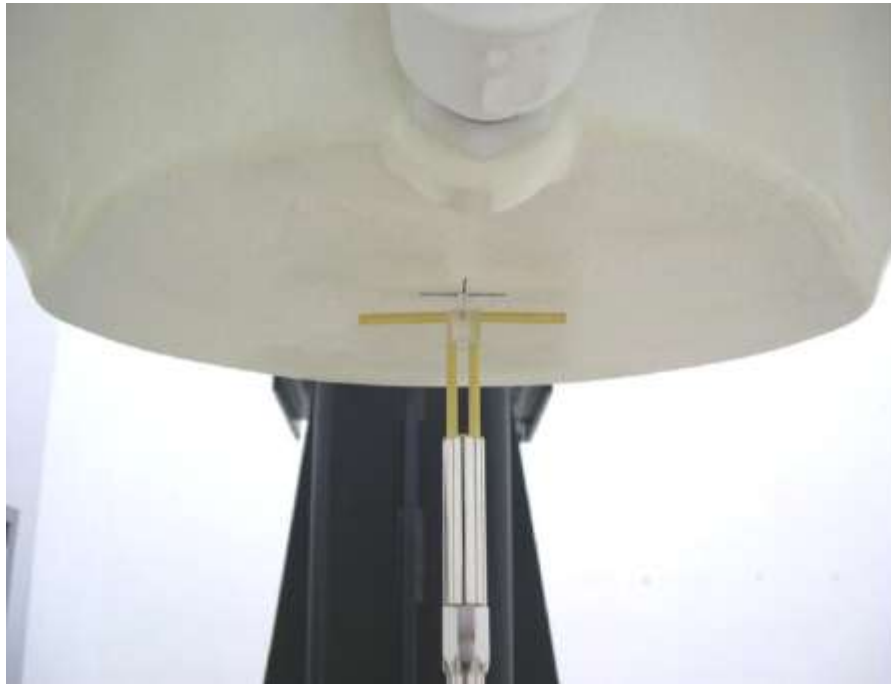
Picture 8.2 Photo of Dipole Setup
