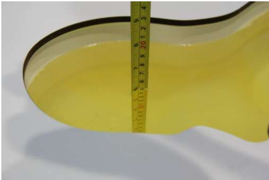
Picture 7-5: Liquid depth in the Head Phantom(2450MHz)
