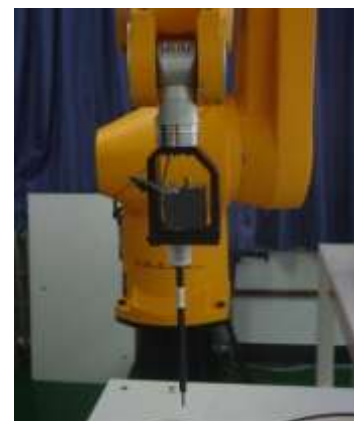
Picture C.3 E-field Probe
