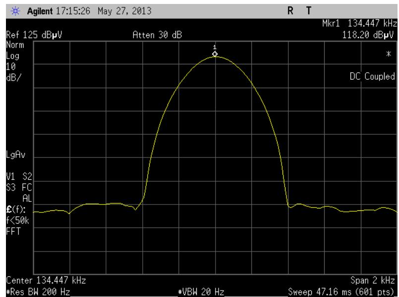
Carrier frequency measured with EUT at +50°C
