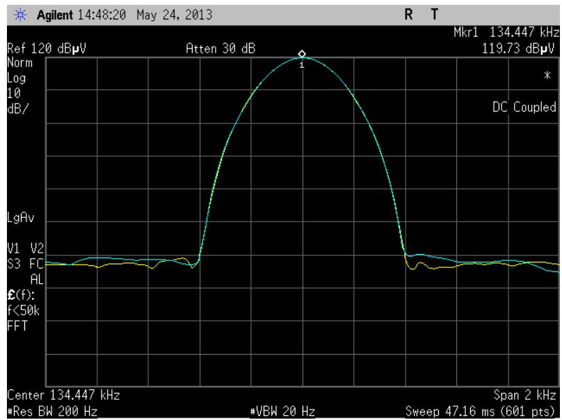
Measures of carrier frequency with the EUT powered at 13.5V at -30°C, +20°C and +50°C
