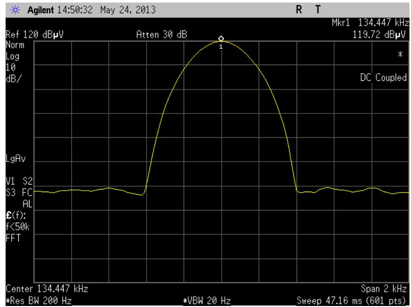
Carrier frequency measured with EUT at -30°C
