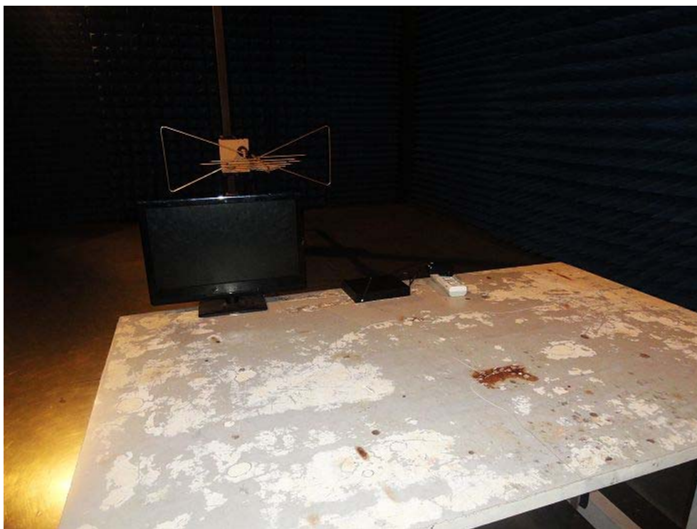
Radiated Emission Test Setup:
