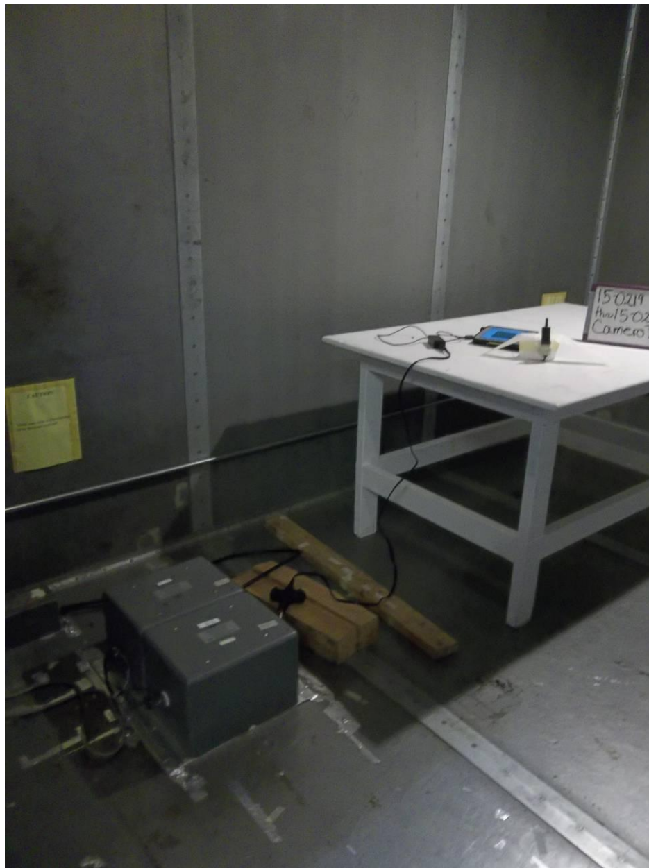
Figure 6. Conducted Power Line Emissions Test Setup
