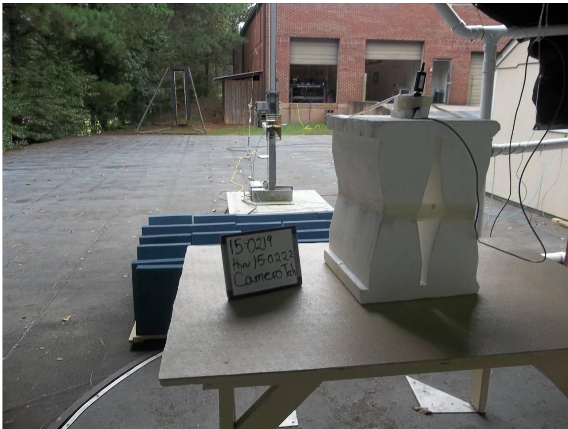
Figure 6. Radiated Emissions Test Setup, above 1 GHz, Back
