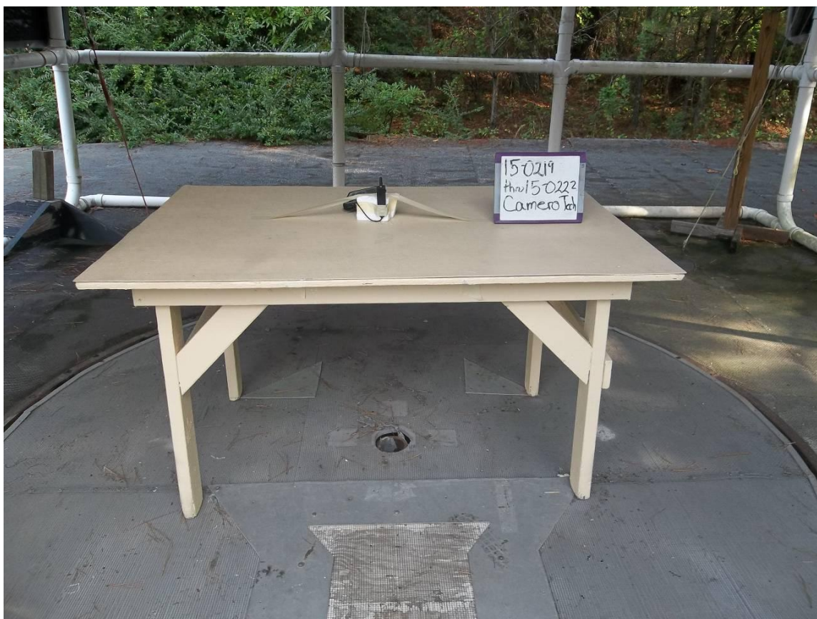
Figure 1. Radiated Emissions Test Setup, Front below 1 GHz
