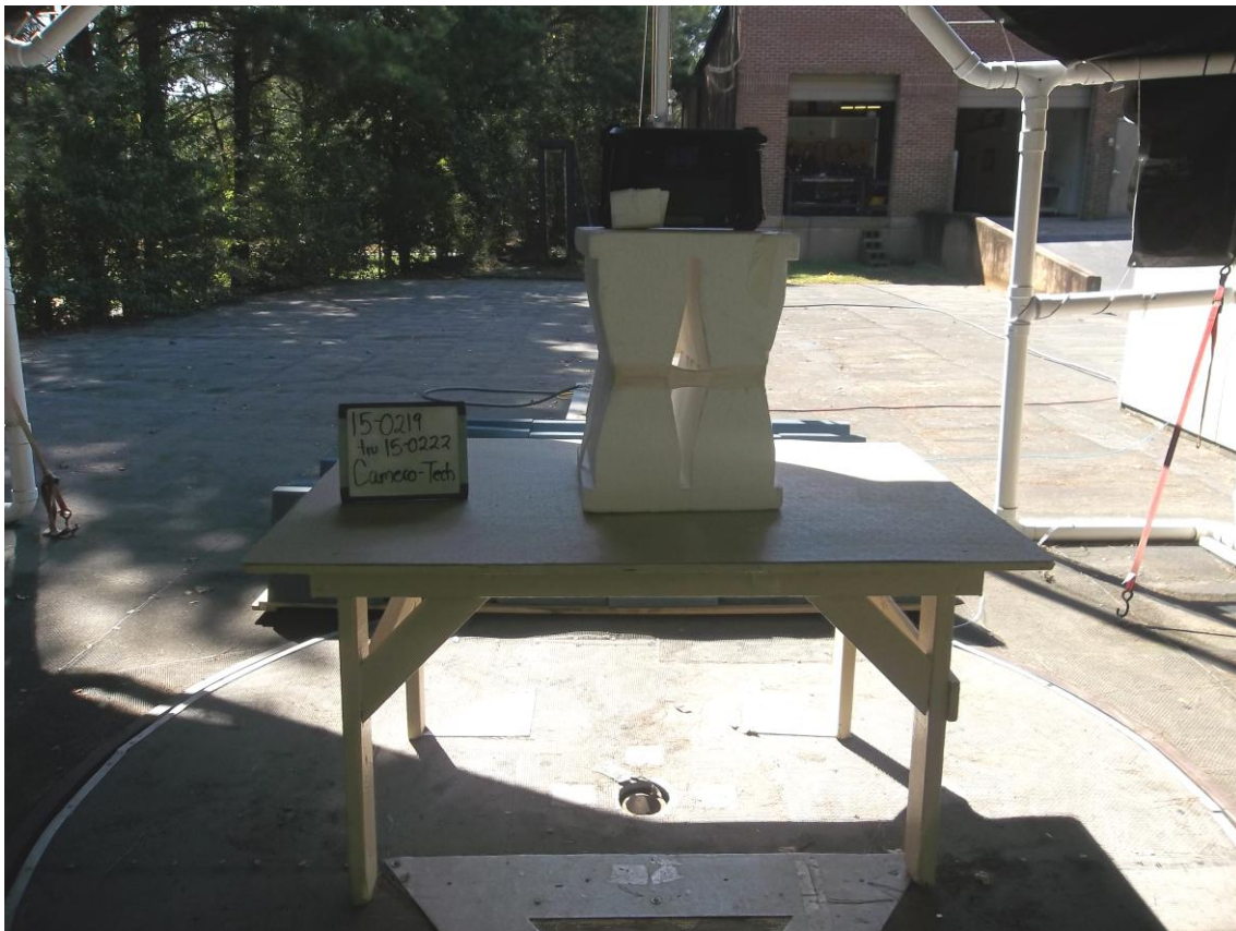
Figure 6. Radiated Emissions Test Setup, above 1 GHz, Back
