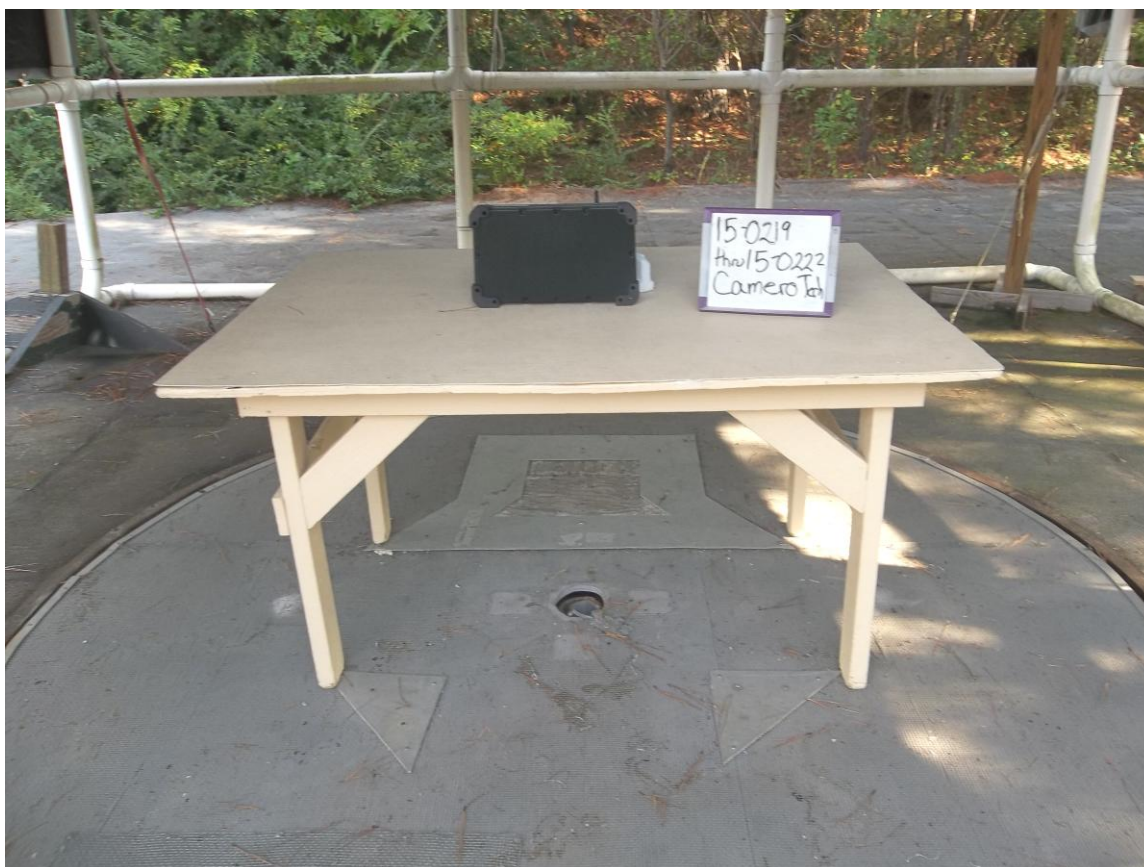
Figure 1. Radiated Emissions Test Setup, Front below 1 GHz
