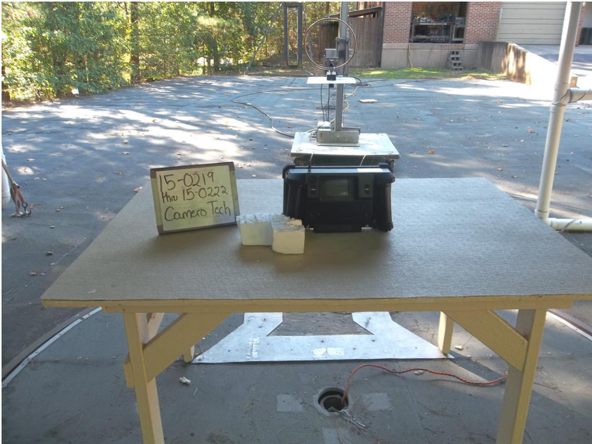
Figure 3. Radiated Emissions Test Setup 9 kHz to 30 MHz, Back
