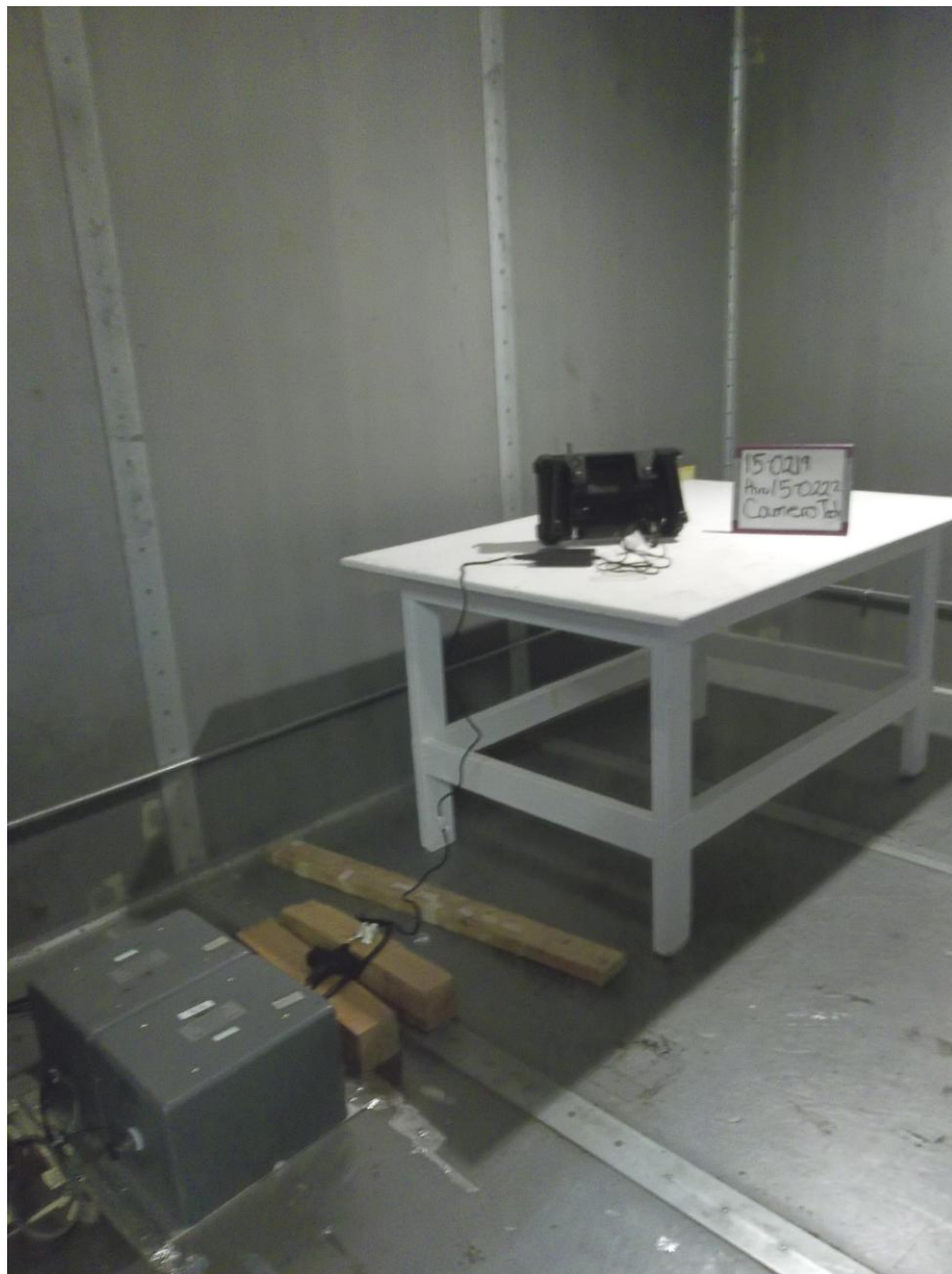
Figure 7. Conducted Power Line Emissions Test Setup
