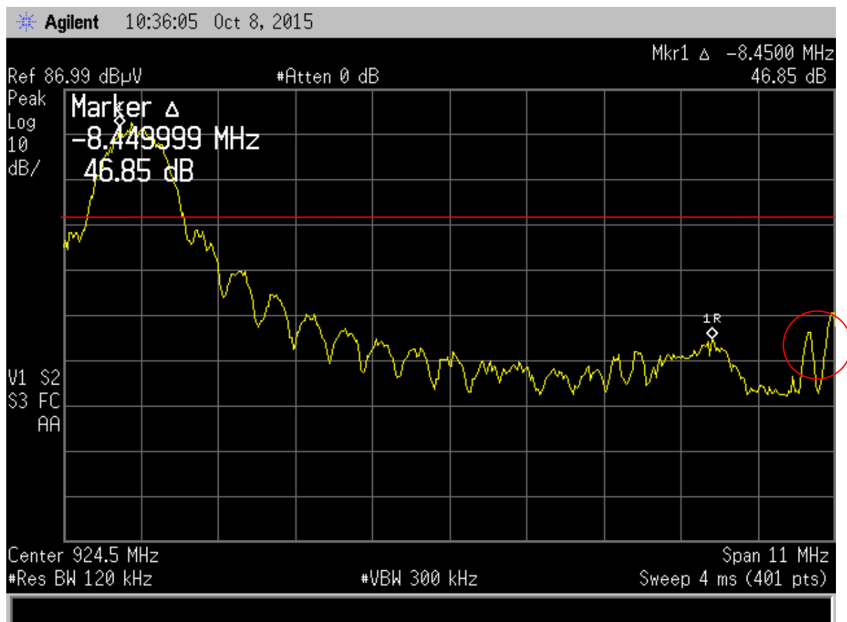
Figure 11. Band Edge Compliance, High Channel Delta – Peak
