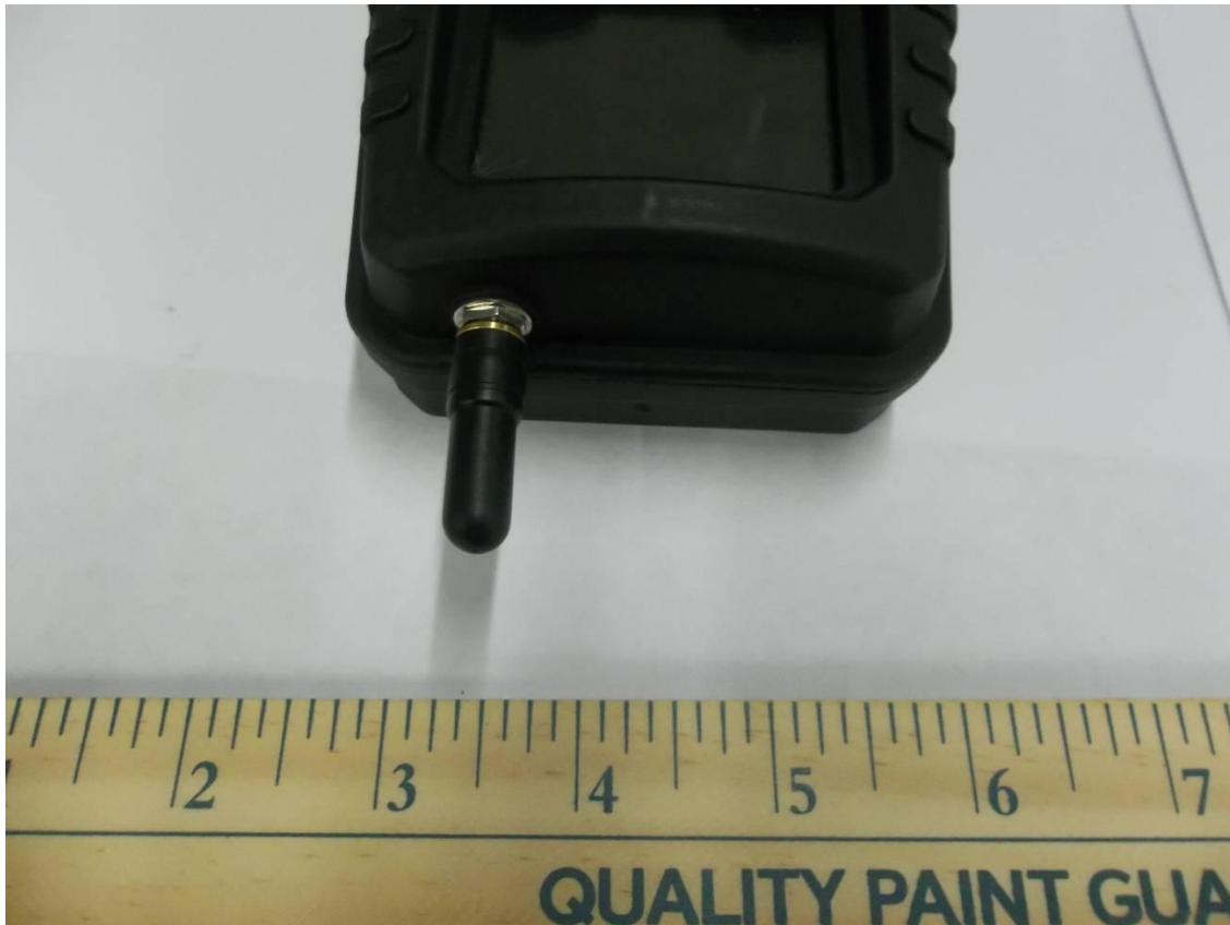
Figure 5. Top of EUT (with Zigbee Antenna)
