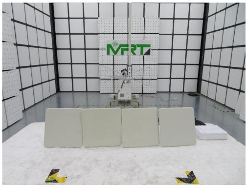
Description: Radiated Spurious Emission Test Setup for below 1GHz For Antenna Configuration 2# (Antenna = 12dBi)
