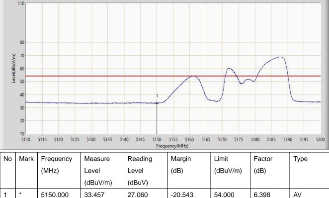
Factor (dB) = Cable Loss (dB) + Antenna Factor (dB/m) - Pre\_Amplifier Gain (dB)
