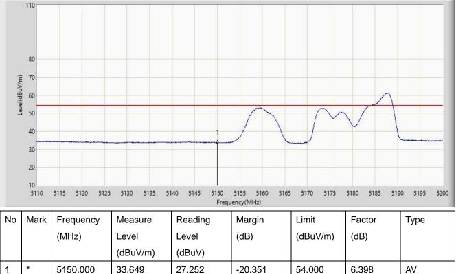
Note 1: Measure Level  $(dB\mu V/m)$  = Reading Level  $(dB\mu V)$  + Factor (dB)
