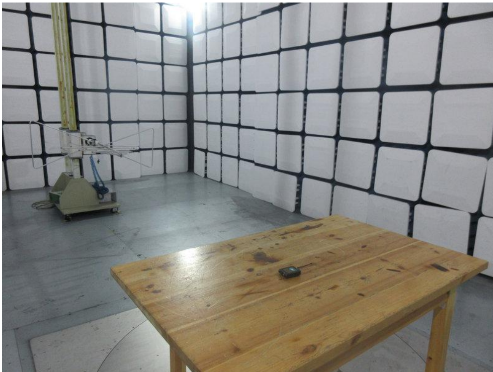
Photo of Radiation Emission Test
