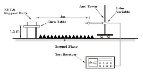
The radiated emission below 1GHz tests were performed in the 10 meters chamber, above 1GHz tests were performed in the 3 meters chamber A, using the setup accordance with the ANSI C63.10-2013. The specification used was the FCC 15.209, and FCC 15.247 limits.
