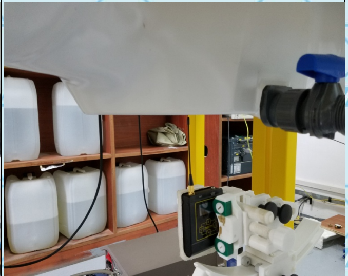
Photo 8: 2450MHz Liquid Depth ≥ 15.0cm
