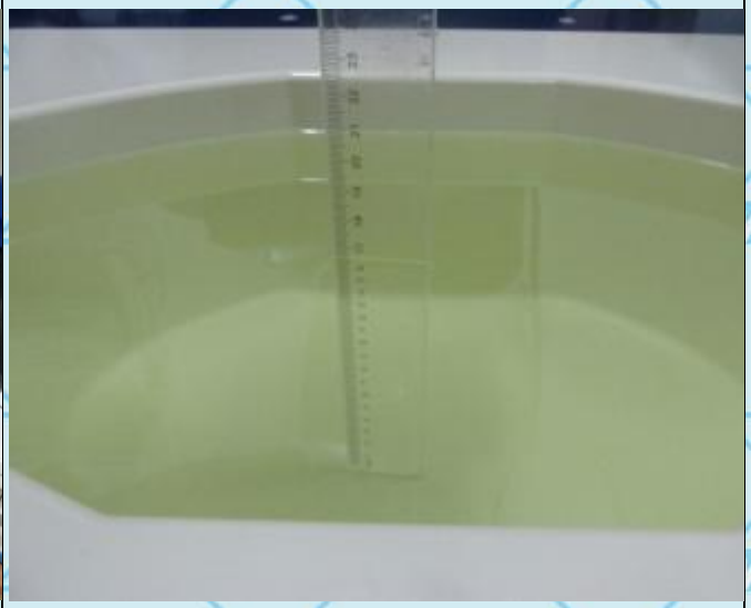
Photo 8: 2450MHz Liquid Depth ≥ 15.0cm
