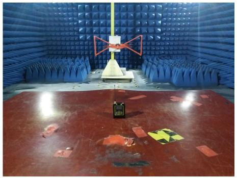
RADIATED EMISSION TEST (Above 1GHz)
