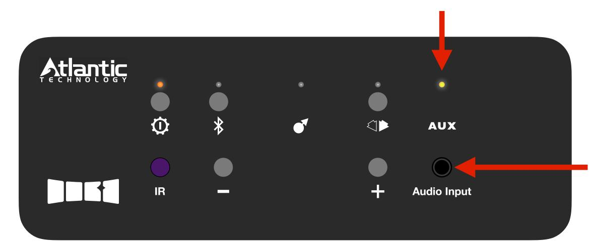
Make sure no cables are plugged into the AUX jack located on the front of the JE-0495. If you want to play audio from the "Line In" input on the back, having something plugged into the Audio Input jack on the front will override the line in audio.
