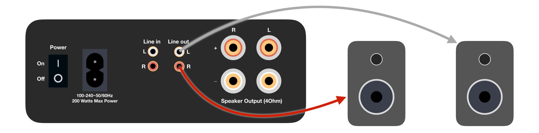
If you are connecting passive speakers (i.e. if your speakers are powered solely by the connection to your STA-200) connect them to the output labeled "Speaker Output".
