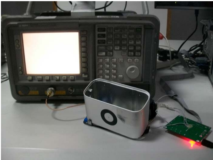
SPURIOUS EMISSION TEST SETUP
